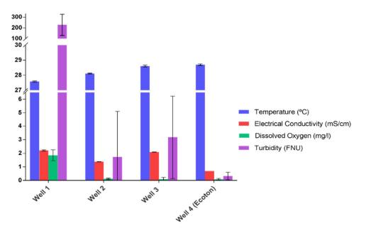
Figure 2 – Scanning of water quality in multiple wells within a village dealing with industry waste contamination.
